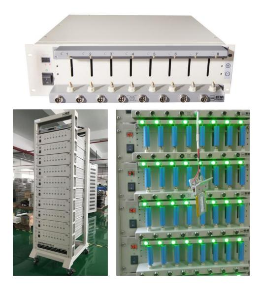
3. BTS4000 For big cells, modules and packs: 5V50A, 5V100A, 20V50A, 50V50A, 60V100A, 100V100A, etc.
